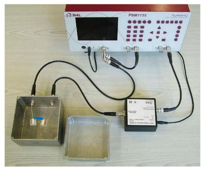
Accessory for use with the PSM1700 or PSM1735 Frequency Response Analyzers for high impedance measurement.
