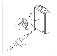
Before securing the inlet wiring in place, the cable clip should be removed. To do this, use a flathead screwdriver and a pivoting motion to slide the clip out. Wire the connector up with reference to the diagram on the rear panel.
