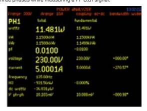
Where users wish to see measured functions at higher resolution, any selected measurements can be viewed with a 6 digit display. Here, we see 6 digit presentation of items selected in the first screen.
