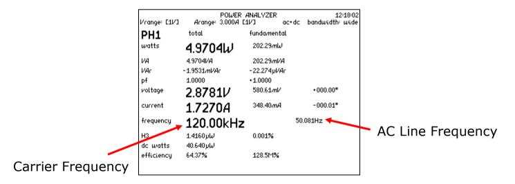
Phase 2 will also display the same two frequency components for the user's reference.
