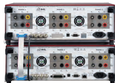
PPA5500 units in Master/Slave mode, synchronised for 4-6 Phase measurements
