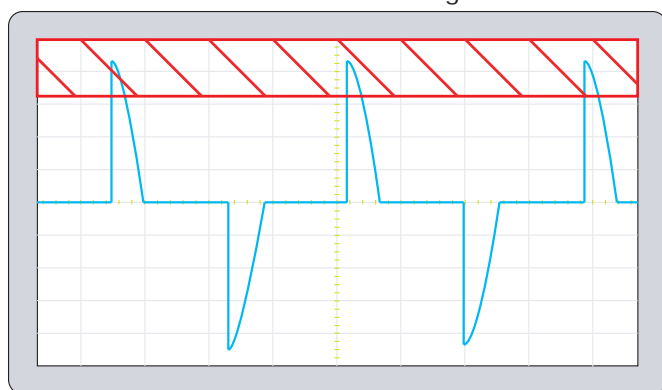
Example RMS Ranging system, commonly used in older instrument designs
