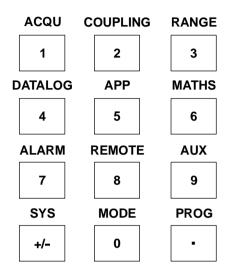
SELECT MENUS for non-mode-specific configuration. Also use as numeric keypad when entering parameter values or data.
