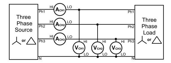
To configure PPA35xx to calculate the correct phase power when the Load topology is in a Star Configuration; Access "Power Analyzer" mode either through the "Mode" or the "POWER" button as per the screenshot below
