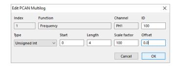
Editing a multilog allows you to change the format type, start location in the message, the length of the message this value will use up and a scale factor and offset. Additionally, if "Send Multilog Data over CAN" is set to "To custom IDs" you can also edit the ID the message will be sent to.
