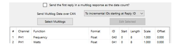
Additionally the ID starts at the CAN Reply ID, and increases each message that will need to be sent across the CAN Network, as "Send Multilog Data over CAN" setting is set to "To incremental IDs starting at Reply ID". Selecting "To the Reply ID" changes the ID value to the CAN Reply ID:
