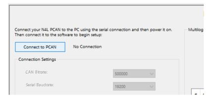
Select serial, the correct com port and the correct baud rate (default: 19200). Use the Test button to check if the software is able to form a connection and communicate with the **CAN-port** unit; once the settings are correct press Connect.
