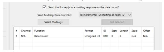
PPA Datalogger will display a wide selection of Multilog parameters, check the values you want to log and then press OK.
