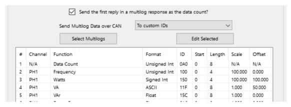
Multiple values can be share a CAN message by ensuring that they do not overlap and fit in 8 bytes. If the "Send Multilog Data over CAN" is set to "To Custom IDs" they also need to share IDs.
