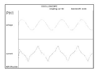
Fig 1 (Distorted current waveform)
