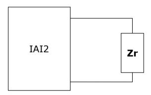
Then, if **ZI** is the impedance measured by the IAI2 with the known reference impedance **Zr** connected and **Zm** is the impedance measured by the IAI2 with the DUT connected:
