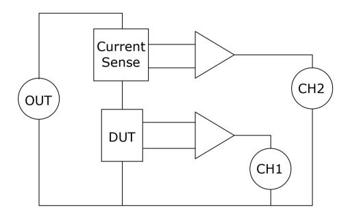
The IAI2 has 4 selectable 'shunts' to sense the current through the device under test:
