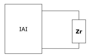
Then, if **ZI** is the impedance measured by the IAI with the known reference impedance **Zr** connected and **Zm** is the impedance measured by the IAI with the DUT connected:
