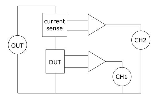
The IAI has 4 selectable 'shunts' to sense the current through the device under test:
