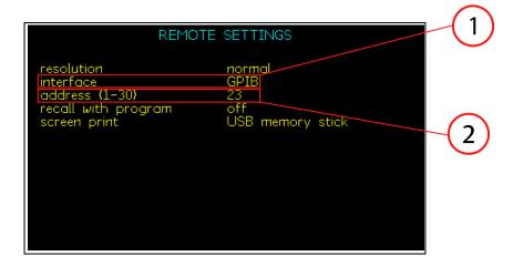
Communication settings are under the remote menu, press the remote key to show available settings. First select GPIB from the interface drop down (1) and press ENTER. The address option (2) will appear, use this to set the GPIB address for your application.
